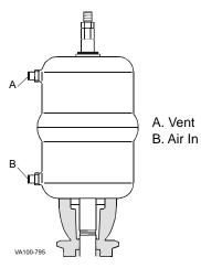
Figure 9: A, B and C Size Air-to-Raise, Maintenance-Free
