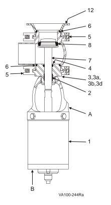
Figure 21: W64R/W84R Tank Outlet Valve
