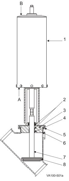
Figure 12: W61Y Shut Off Valve
