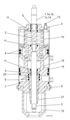
Figure 38: 4" Air-to-Raise 3-Position Actuator
