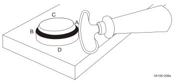
Figure 31: Pressing Tri Ring Into Plug
