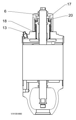
Figure 41: 4", 5", and 6" Air-to-Raise, Adjustable-Spring Actuator
