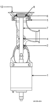
Figure 22: W64ET Tank Outlet Valve
