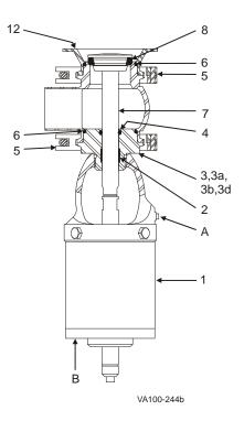
Figure 19: W64/W84 Tank Outlet Valve
