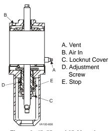
Figure 8: 4", 5", and 6" Air-to-Lower, Adjustable-Spring
