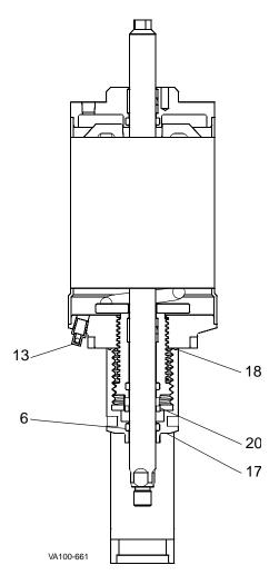
Figure 42: 4", 5", and 6" Air-to-Lower, Adjustable-Spring Actuator
