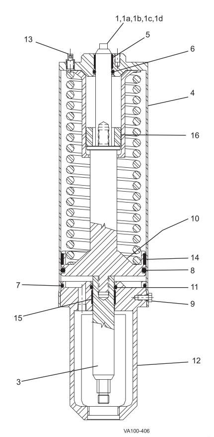
4" and 6" Air-to-Spring Long Stroke Actuator
