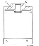
Figure 35: Remove O-ring and Bearing
