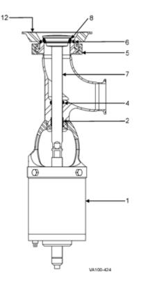
Figure 23: W64ET Tank Outlet Valve
