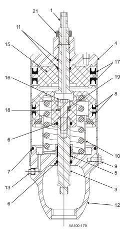
Figure 39: 4" Air-to-Lower 3-Position Actuator
