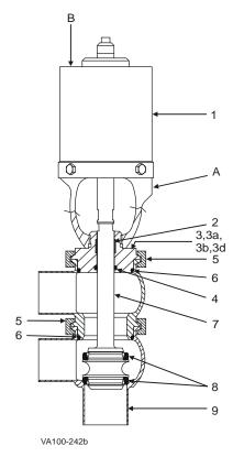
Figure 15: W62/W82 Divert Valve (Air-to-Raise Shown)
