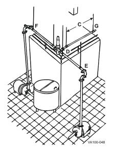
Figure 1: Pipeline Support
