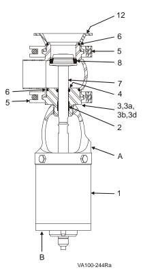
Figure 20: W64R/W84R Tank Outlet Valve
